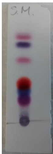
Figure A5.1 Silica TLC plate showing the separation of the 6 components of the reaction mixture of formazan 5.7 with \text{BF}_3 \cdot \text{OEt}_2 and \text{NEt}_3 .
